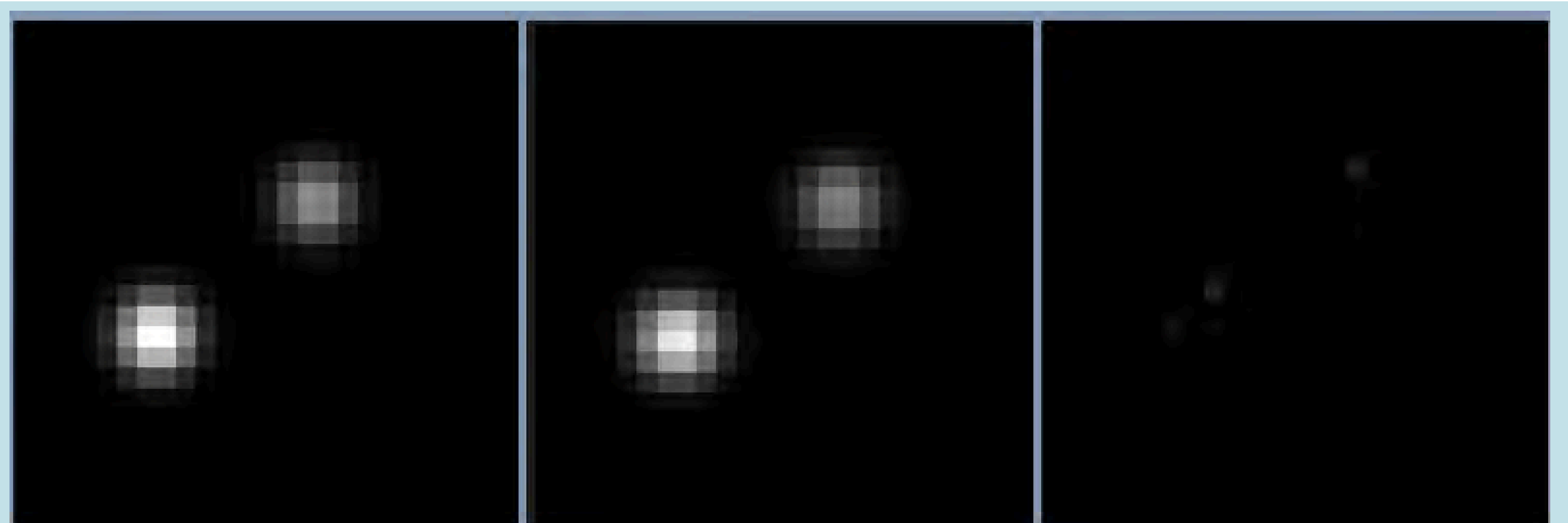
Fig. 3 - Simulated image of two stars using an empirical Gaussian PSF model. Starting from left to right we show the two-star simulated image, the six-parameter best fit we calculate and finally the residuals of the best fit solution (Reksini in prep.).
